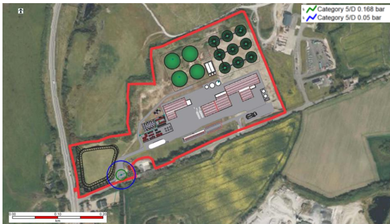
Figure 6-18 Below Ground Biogas Pipeline Rupture (Horizontal) and VCE: 1% Fatality Outdoors and 1% Fatality Indoors CIA. 3 Contours
